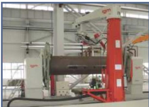
CNC gas cutting machine for plate cutting ensures precision cutting of shell plates and profile cut tube plates.
