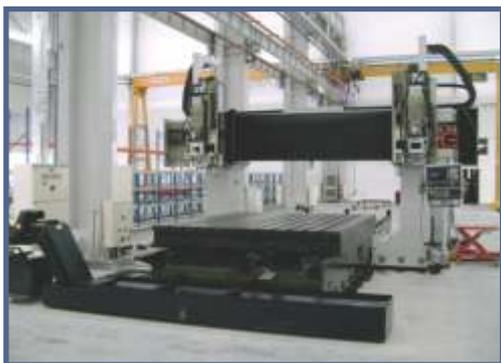
CNC twin spindle drilling machine with high speed and direct feed technology ensures fine tube hole finish and accuracy, which is important for leak tight expansion and effective heat transfer.
